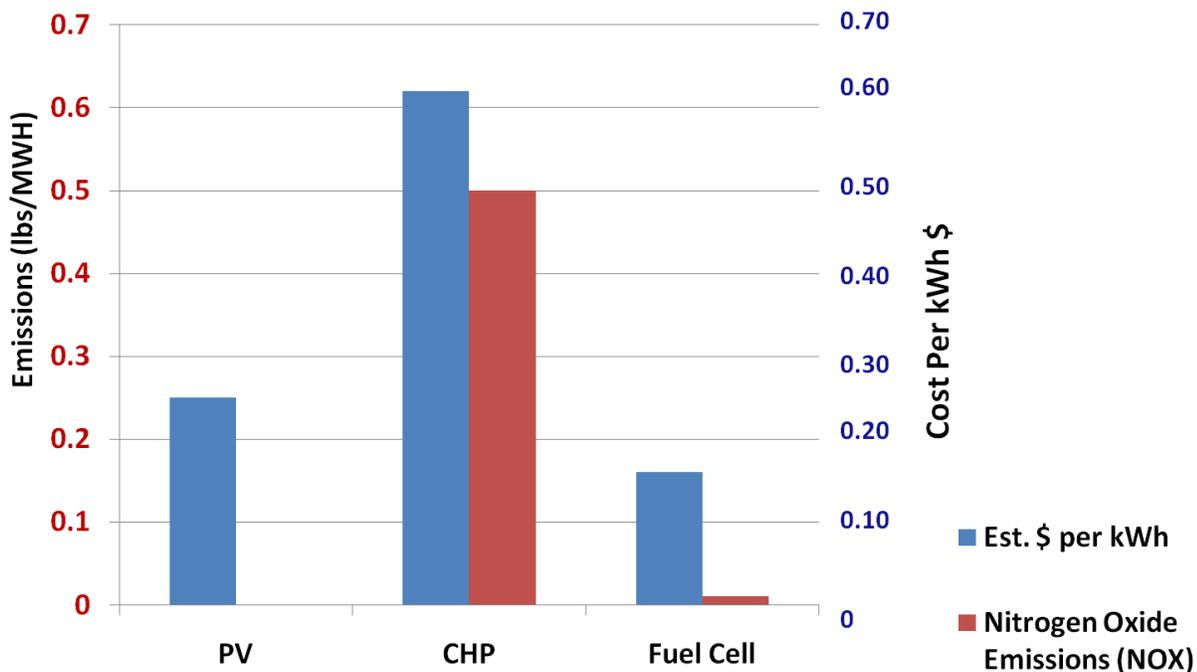
This graph illustrates the cost per kilowatt hour and the nitrogen oxide emissions of the three systems. The system costs per kilowatt hour can be found on the right side of the graph. The emissions of Nitrogen Oxide for each System can be found on the left. Each system weighs in differently.
