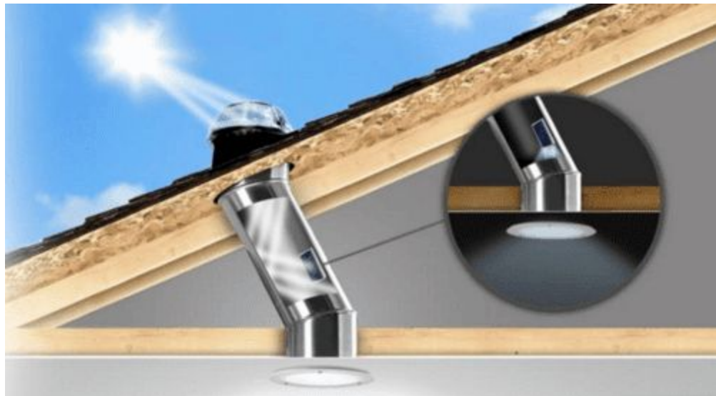
Tubular skylight cross-section.
