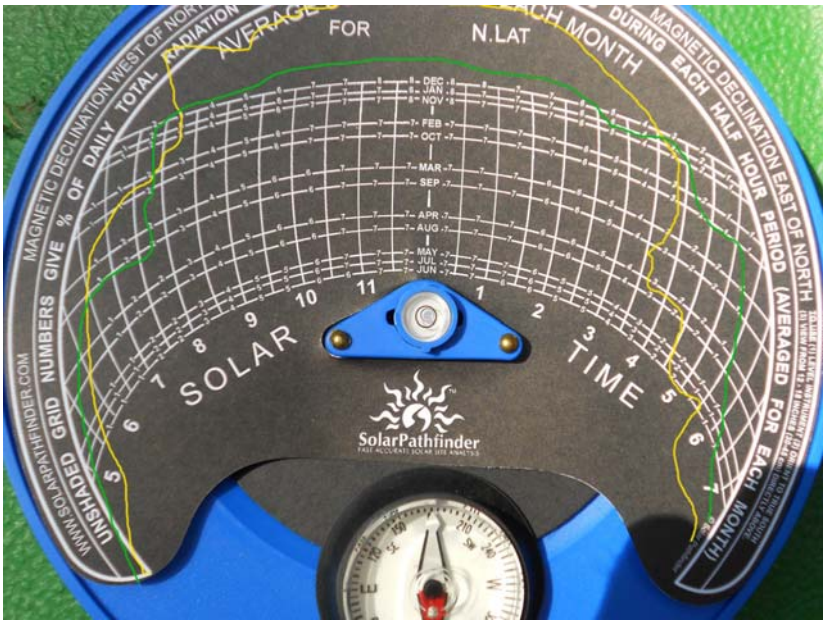
Figure 4: Solar Pathfinder tool used to collect available sunlight locations on the recreation center’s roof. The yellow line represents the East side of the building; the green line represents the west side of the building. Any area inside the lines is available sunlight.
