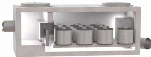
Example of a stormwater vault
