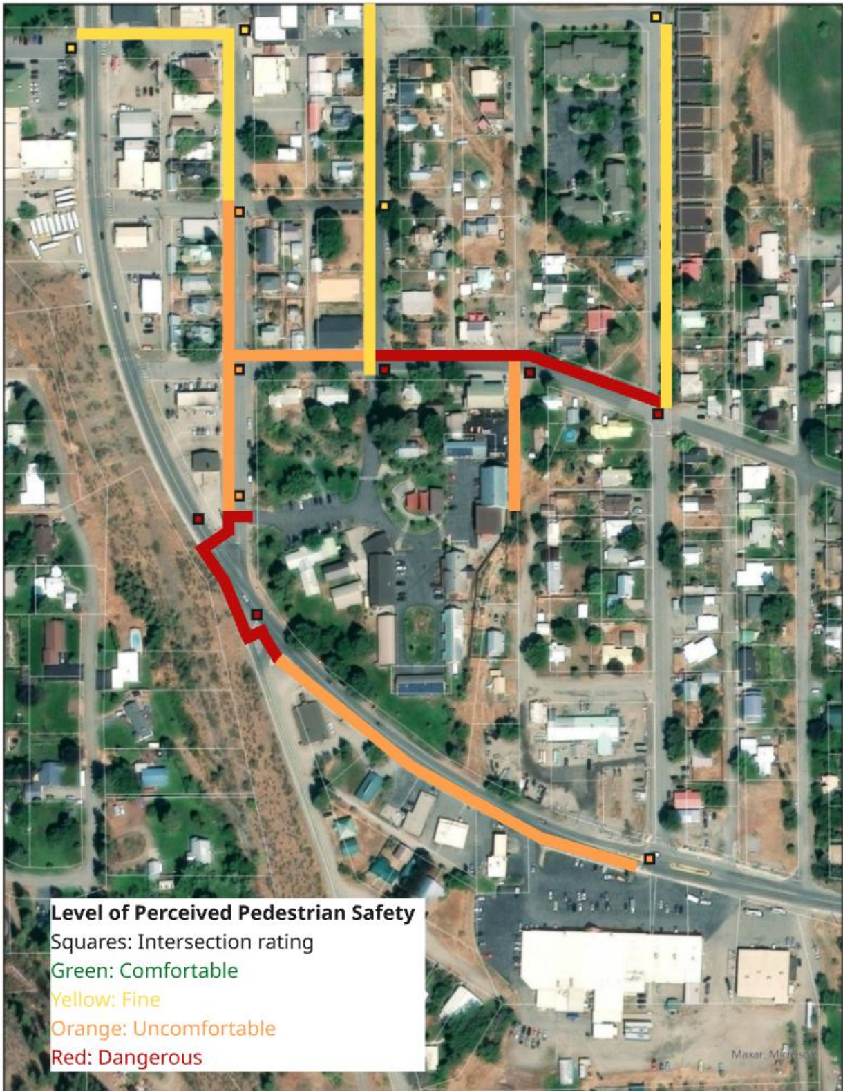
Figure 28 Map of routes and their level of perceived pedestrian safety, created by our team
