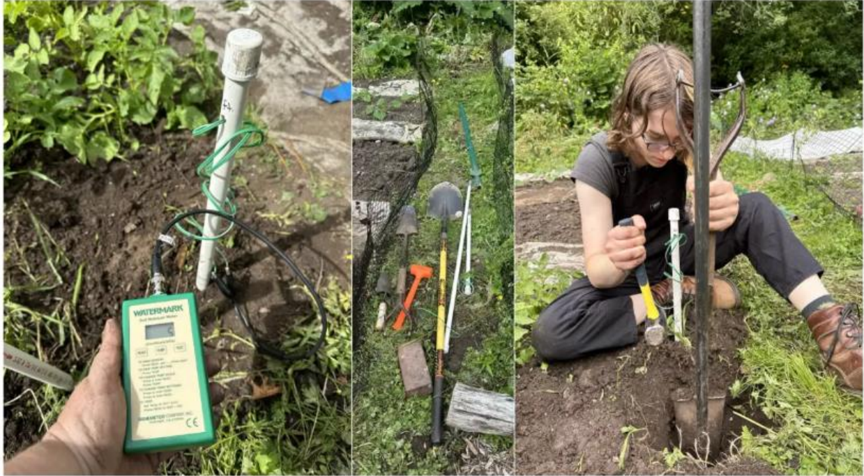
Pictured: (L) installed moisture sensor and current reading; (M) tools for installing sensors; (R) Outback farmer Skye Schultz installing moisture sensors. Source: Outback Farm
