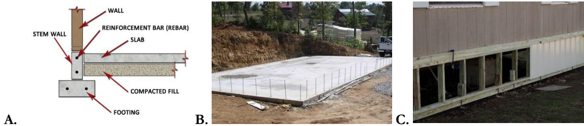
Figure 2. A diagram showing a stem wall (A) (“Stem Wall Foundation,” n.d.), a slab on grade foundation before it has been built on (B) ([Concrete Slab Foundation], n.d.), and a pier and beam foundation partially covered by a skirt (C) (Green Building Advisors, n.d.).
