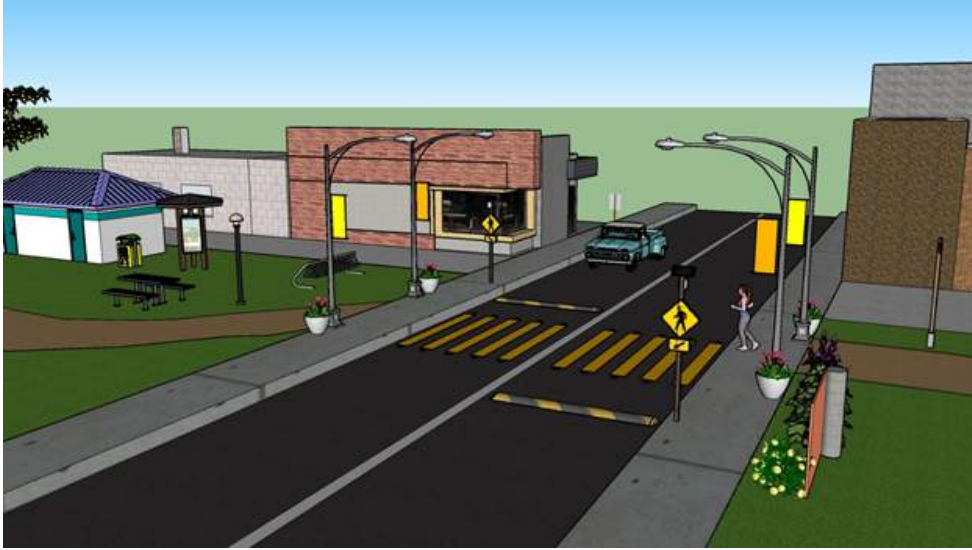
Figure 10. Recommended crosswalk safety improvements that could be made along the Centennial Trail in Arlington
