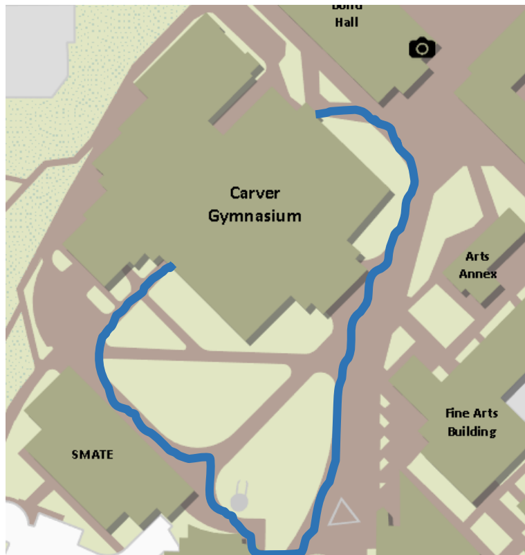
Figure 6 Blue Line = Assumed irrigation perimeter for SMATE water meter.
